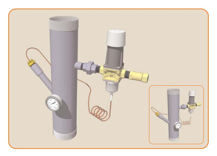
The Cemline After Cooler assembly mixes hot water with cold water resulting in liquid temperatures acceptable for municipal sewage and per the local code. This packaged after cooler is perfect to be installed after a flash tank, blow down tank, or condensate receiver as condensate should be flashed before entering the condensate after cooler.
