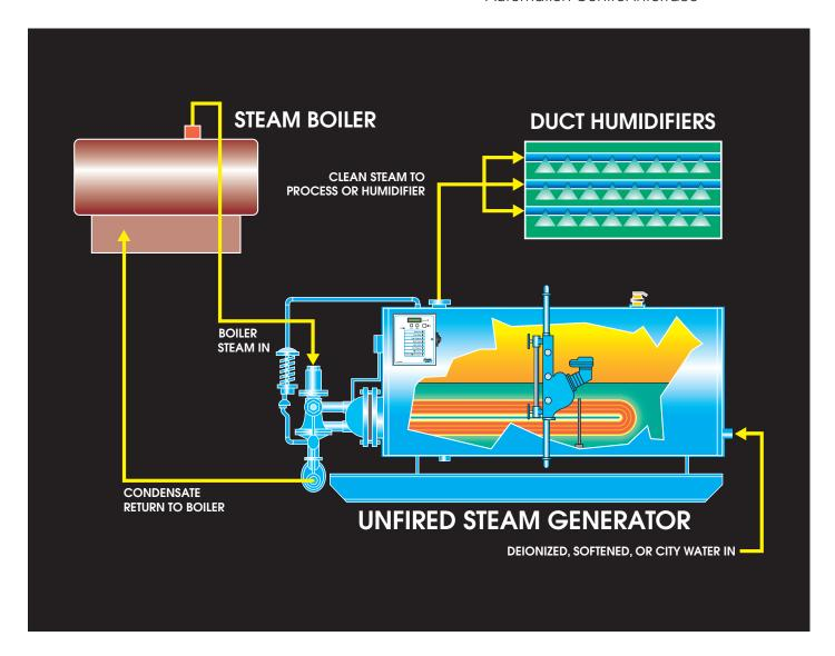
Cemline Corporation is the industry leader for Unfired Steam Generators with leading edge sizing software, application knowledge, and advanced technology. As a standard Cemline supplies features including control valve, level controls, feedwater solenoids, steam separator, and a solid state control panel with contacts indicating functions and alarms for the Building Automation Systems (BAS).
