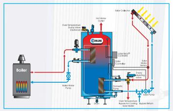
Feed-Forward Water Heater - FFH Series - The Cemline Steam Fired Feed Forward Instantaneous Water Heaters use a pressure sensing blending valve to mix overheated hot water with cold water to make hot domestic water. Cold water is passed through the tubes of the heat exchanger while 2 to 15 psig steam is piped to the shell of the heat exchanger which overheats the water in the tubes. A differential pressure sensing head control valve
