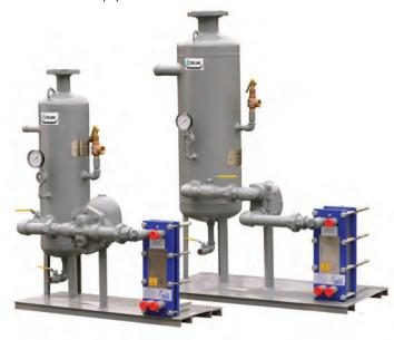
Blow Off Tanks - BOT Series - are vessels used as holding tanks to reduce the pressure and temperature of water drained from boilers and to ensure the safe release of boiler drain water into the sewage system.
