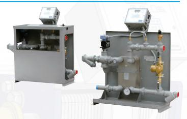
Solar Water Heaters - SLR Series - use solar energy from an external solar collector or can be dual energy source unit using either boiler water, steam, or electric as the back-up energy source for times when solar energy is not enough or unavailable. The solar water heater uses a double walled brazed plate heat exchanger to maximize heat transfer between the solar and the domestic waters.
