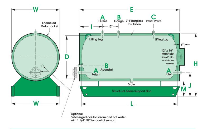
\* For Submerged coil sizing, see Cemline Submerged Heating Coil catalog section or go to www.cemline.com for Automated Sizing Program.
