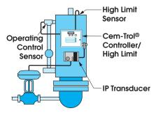
An air-operated valve can be used with either steam or hot water as the heating medium. Air operated valves are normally used in buildings when building control air is available.
