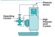
**(Energy Source-Steam):** A pilot operated steam control valve uses a steam pilot to monitor output steam pressure and automatically modulate the flow of source steam to maintain a constant output steam pressure. A pilot operated controller is field adjustable.
